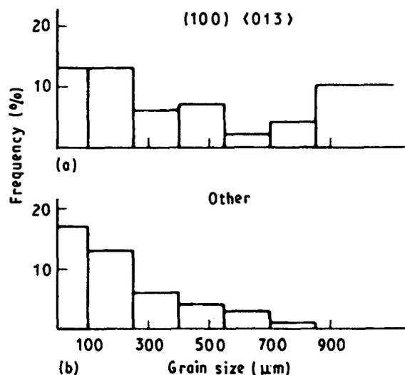
Figure 15 EBSD-determined microtexture of an Al-SiC composite shown as frequency histograms of grain sizes of grains having microtexture (a) close to  $\{100\}\langle 013\rangle$ , and (b) all other microtextures. (Courtesy Juul Jensen *et al.* [50].)
