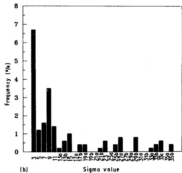
Figure 18 Frequency histogram of  $\Sigma$  values for CSL boundaries in annealed nickel as determined by EBSD. The CSLs on Fig. 17 are a subset of these data; (b) Represents a specimen which has undergone a longer anneal than (a) and has a sharper mesotexture.
