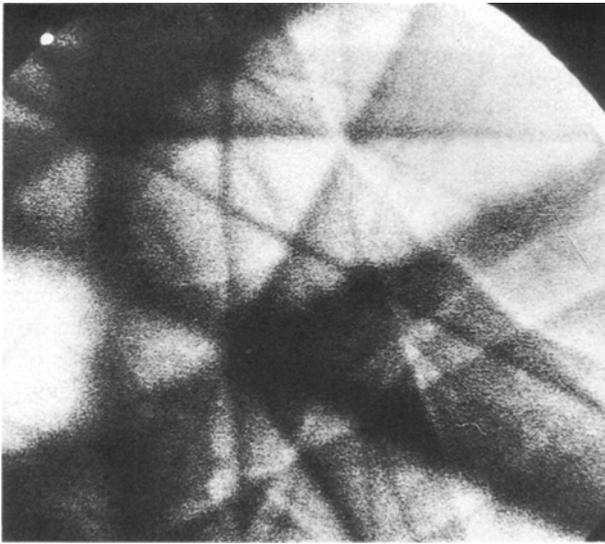
Figure 3 An example of a selected-area channelling (SAC) pattern.
