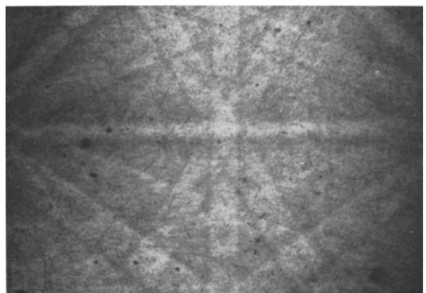
intensity of each pixel is determined. The Hough transform maps each pixel onto a curve in Hough space each point on the curve being assigned an intensity equal to that of the pixel. The equation of the curve is
